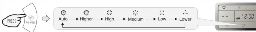
**!At "FAN ONLY" mode, the "AUTO" is not available. At "DRY" mode, fan speed is set as "AUTO" automatically, "AFN" button is ineffective in this case.**
