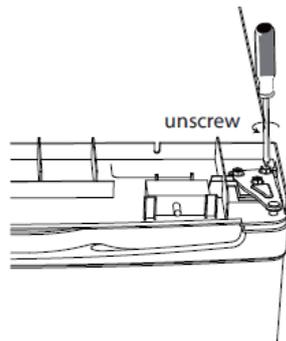
4.Remove the screws and bottom hinge. Then remove the adjustable feet from both side.
