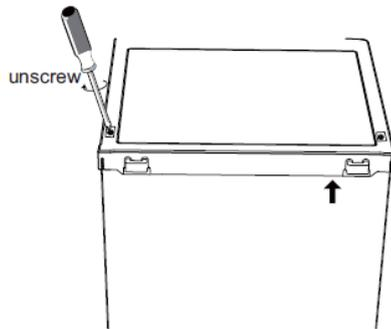
2.Carefully lift the top cover 5cm away from the freezer, then pull out the terminal. Then remove the top cover away.
