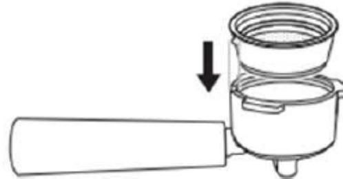
2. Turn the filter to the left or right to lock in place. This will help secure the filter in the porta-filter.
