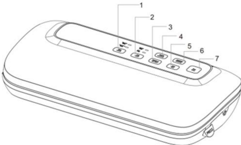
1. **"Mode" button:** it has two setting mode (Normal and Gentle). The default mode is Normal. When the food is crumbly, you can press the button, then the vacuum mode is changed to Gentle. You can manually control the degree of vacuum by pressing "Seal" button at any time, the food will be sealed automatically. (Note: if the power is interrupted, this setting will return to a preset standard mode)
