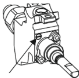
Surub de bypass
