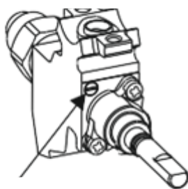
Surub de bypass
